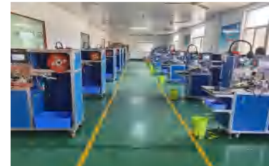
Fully Automatic Core Winding Machines (24 Units)
